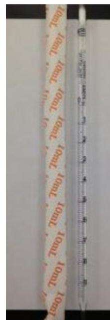
Figure 5. Graduated pipettes for transfer of liquids
