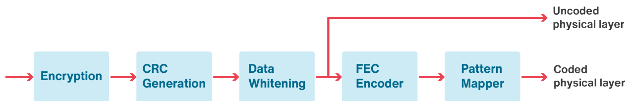
Figure B.3: Transmitter bit data path for un-coded 1M and 2M physical layers in BLE 5
