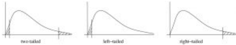
Figure 9.5 : Schematics of the critical regions for \chi^2 tests of variance. In the two-tailed situation the tail areas are equal.
