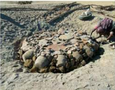
Figure 19 Pottery kilns in Jabarūna village in the form of a pit with metal shreds and plates at the top as isolation to protect vessels from the flames and different stages of the firing preparation
