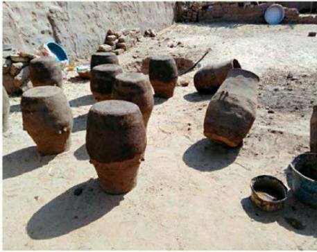
Figure 18 Process of drying in the courtyard of the potter's house (top) and vessels with a yellow burnishing surface ready for firing (bottom)
