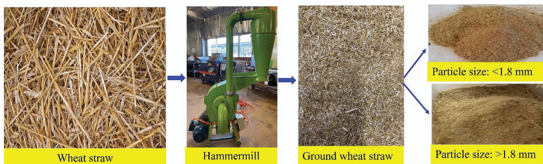
Figure 1. Size reduction of wheat straw for pelletizing.
